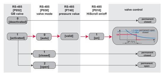
Fig. 7: Pressure-dependent gas ballast valve control in automatic mode
