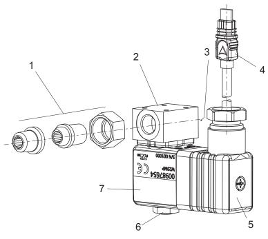
Fig. 2: Design of the solenoid valve for gas ballast valve
