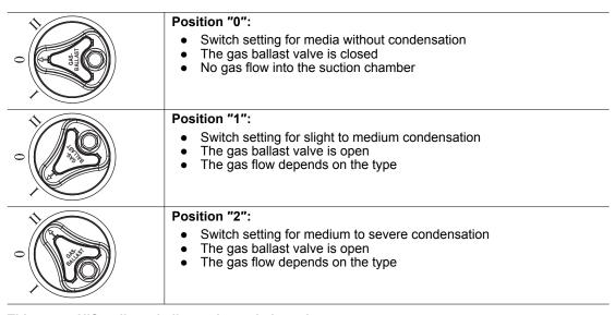
Tbl. 5: HiScroll gas ballast valve switch settings
