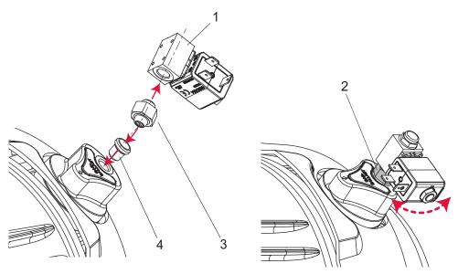
Fig. 4: Installing and aligning solenoid valve
