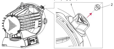
Fig. 3: Preparing gas ballast valve
