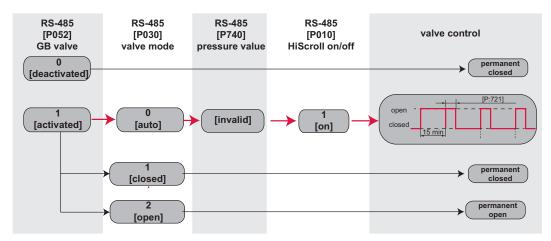
Fig. 8: Gas ballast valve control in automatic mode
