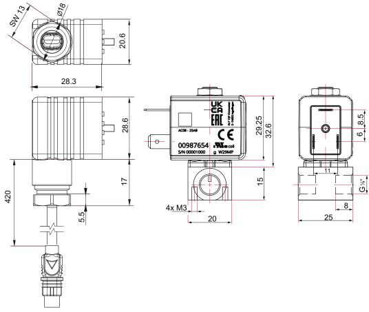
Fig. 9: Solenoid valve dimensions
