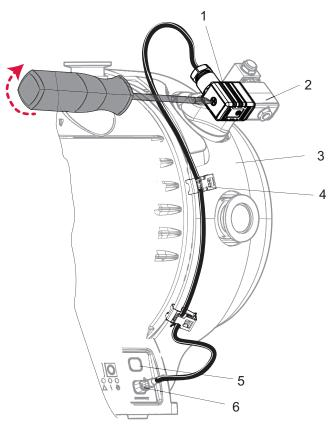
Fig. 5: Electric connection of solenoid valve
